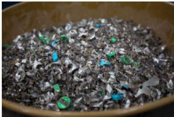
Lighting waste is crushed and separated to recover the mercury.
